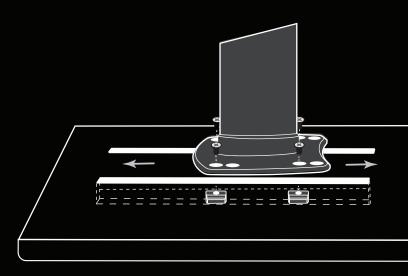
IMPORTANT NOTE: When getting started with the Hover Glide FSURF, we recommend mounting the foil as far back on the board as possible until you get a feel for your new setup. This means using the front hole pattern on the pedestal and sliding the track as far back as possible. This is the most balanced position for this foil/board combination, particularly when riding with footstraps. We highly recommend this position until you gain the experience and confidence necessary to try other locations.
