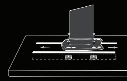
IMPORTANT NOTE: When getting started with the Hover Glide Fwake, we recommend mounting the foil as far back on the board as possible until you get a feel for your new setup. This means using the front hole pattern on the pedestal and sliding the track as far back as possible. This is the most balanced position for this foil/board combination, particularly when riding with footstraps. We highly recommend this position until you gain the experience and confidence necessary to try other locations.
