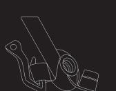
To close purge valve, push in cap and secure velcro straps from bottom to top.
