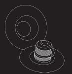
Step 3. Secure the valve cap back in place and re-attach the valve velcro cover.
