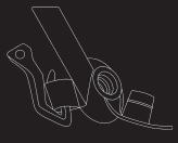
To close purge valve, push in cap and secure velcro straps from bottom to top.
