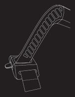
Step 2. Check to make sure handle base is fully seated in the handle mount. To release, press down on tab and pull.
