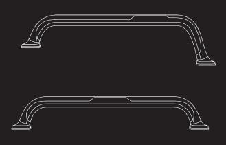
The top Handle mounts on the front of the wing while the bottom one mounts in the rear.
