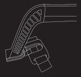
Step 1. Slot the base of the handle clip into the handle mount.
