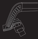
Step 1. Slot the base of the handle clip into the handle mounts on the outer mounting points of the wing. Installation of the handle while wing is defated is recommended.
