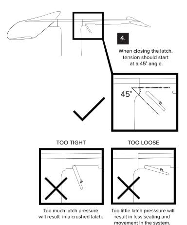
Note\* During the first use, close, open and tighten latch 4 times to properly stretch the Dyneema line and learn about how to adjust the system.
